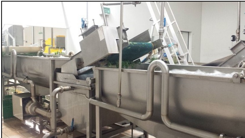
Photo 1. Example of bubble washing system used for washing.
