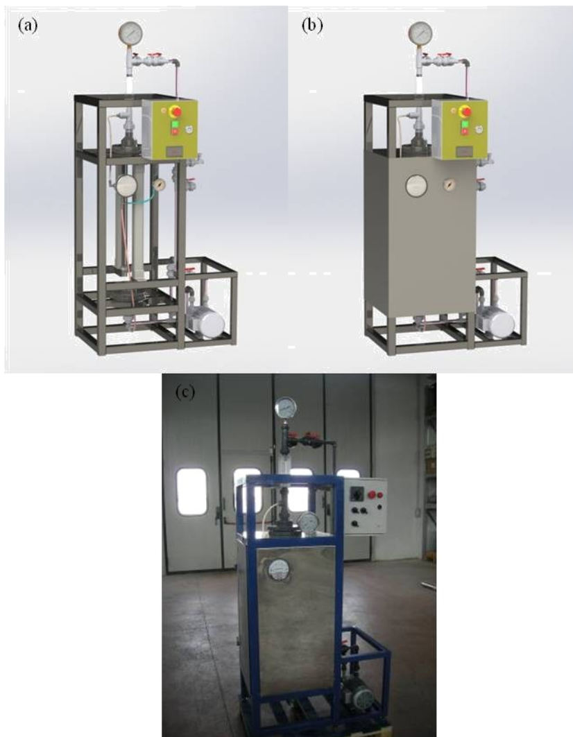
Figure 7.1.4. Rendering (a and b) and a photo (c) of the fluidized bed photocatalytic reactor prototype (STC s.r.l.).
