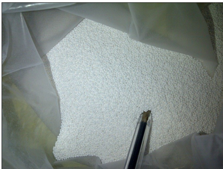
Figure 7.3.1. Alumina microspheres sample
